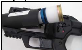
Fig. VI - Install discriminator in weapon using unloaded adapter shell
