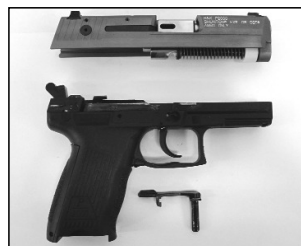
Fig. IV Disassembled pistol ready for conversion
