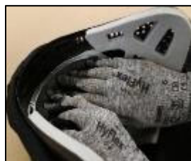
Fig. 18b - FX® 9003 Goggle Assembly top foam verification
