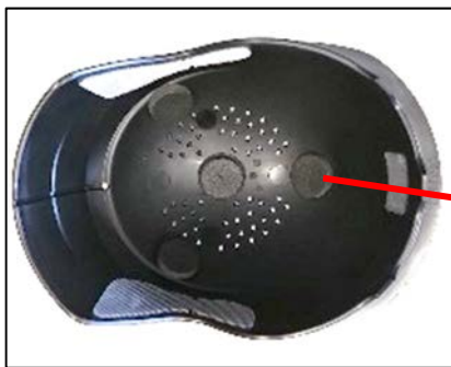
Fig. 8 – Hard top cover, inside view
