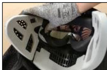
Fig. 18c - FX® 9003 Goggle Assembly bottom foam verification
