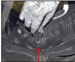
Fig. 23 – Face shield marked center line at the chin area
