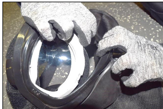
Fig. 42a - Nose portion of the FX® 9004 Helmet, Head Protector's plastic shell
