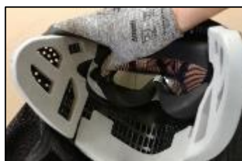
Fig. 18c - FX® 9003 Goggle Assembly bottom foam verification
