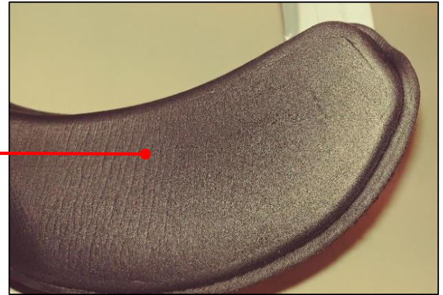
Fig.: 2a - FX® 9003/9004 Close Cell Foam enlarge view of soft surface finish
