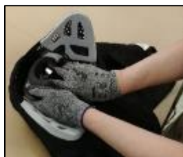
Fig. 13a - FX® 9003/9004 Goggle Assembly side foam verification
