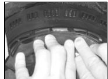
Fig. 12 Goggle frame inside the notch
